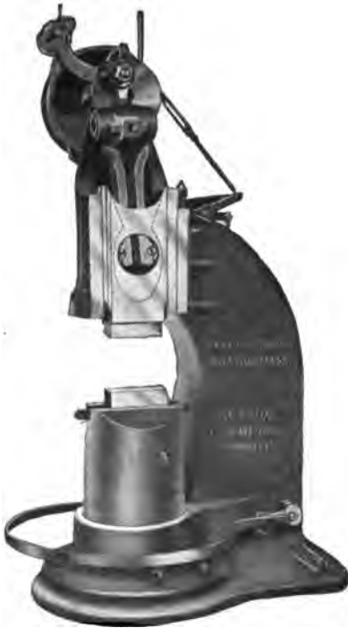
Fig. 22. Beadry Spring-Ram Power Hammer Courtesy of Beadry & Company, Boston, Massachusetts
